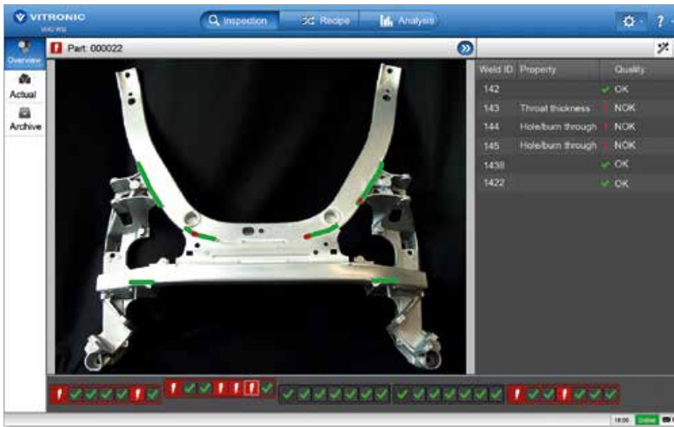
Worker view: clear defect visualization in live operation
