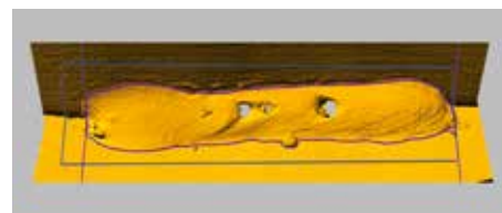
Fillet weld with pores: 3D visualization for workers
