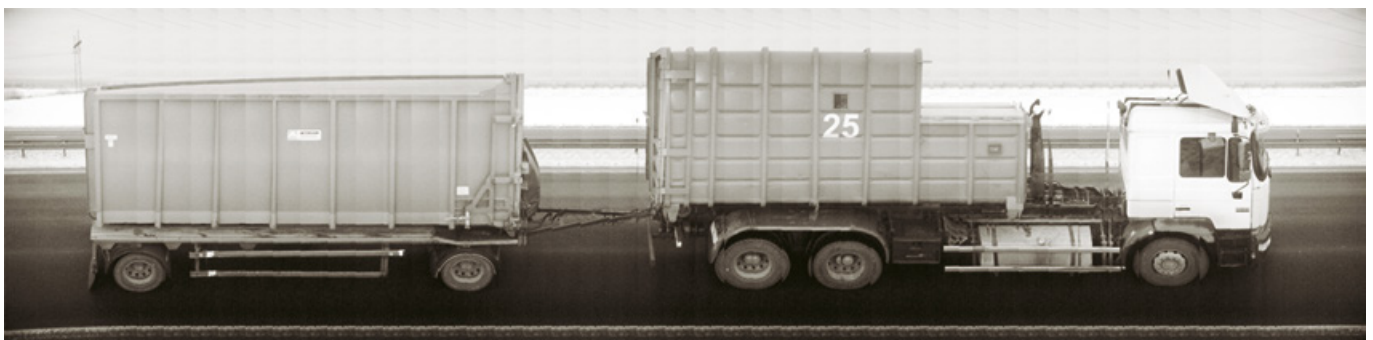
High-res sideways images for classification including size, type, axle count and trailers
